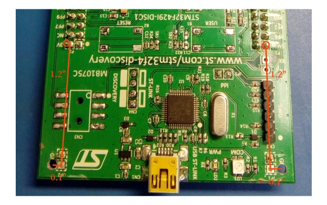
These holes should not cause the mounting screws to come into contact with any signals besides GND. (To be extra safe you could use M2 nylon screws but I did not.)
